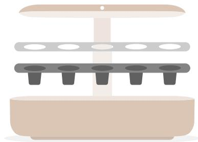
4 Add 2.8L or 0.75 Gallons of water to your reservoir—we recommend referencing the 'Max Fill Line' found on either side of the pump inside the reservoir.
